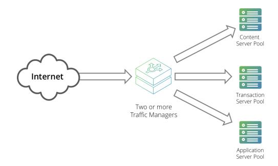
You can install two or more Traffic Managers in a clustered configuration to provide full fault-tolerance for individual software failures. A typical configuration contains at least two Traffic Managers, and at least two servers hosting the load-balanced application.
