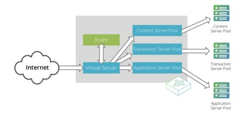
A pool is a collection of nodes. Each node corresponds to a back-end server and port, such as server1.mysite.com:80. You can set up several pools with nodes in common.
