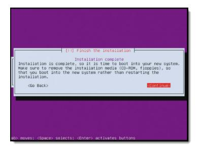
To complete the installation and shut down the appliance, select **Continue** and press Return. Your Traffic Manager is now ready for initial configuration.
